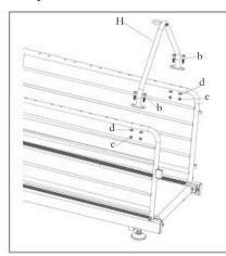
Assemble front hooker rack set (H) onto metal guard rails with the hex screw, curved washer and Nylock (b,d,e)as left figure showing.
