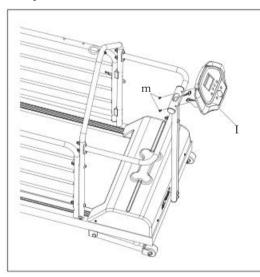
Well connect control cables with Computer assembly (I). Then put the Computer (I) and tighten Console welding assembly with the Truss phillips self tapping screw (m) as left figure showing.
