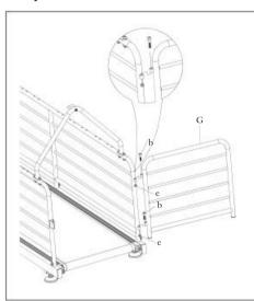
Assemble rear cage door set(G) with right guard rails (E) with the hex screw and Nylock (b,e) as left figure showing.
