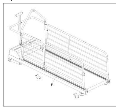
Assemble Metal guard rails (left) + front cage door (F) onto frame by hex screw and curved washer (a,d) as left figure showing.
