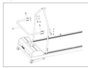
Assemble Reinforced front bar (C) but not tighten, screw tightly by hex screw, curved washer and Nylock (b,d,e) as left figure showing.
