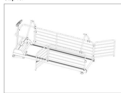
Now finish assembly, the front rails door and rear rails door can be can opened as options.
